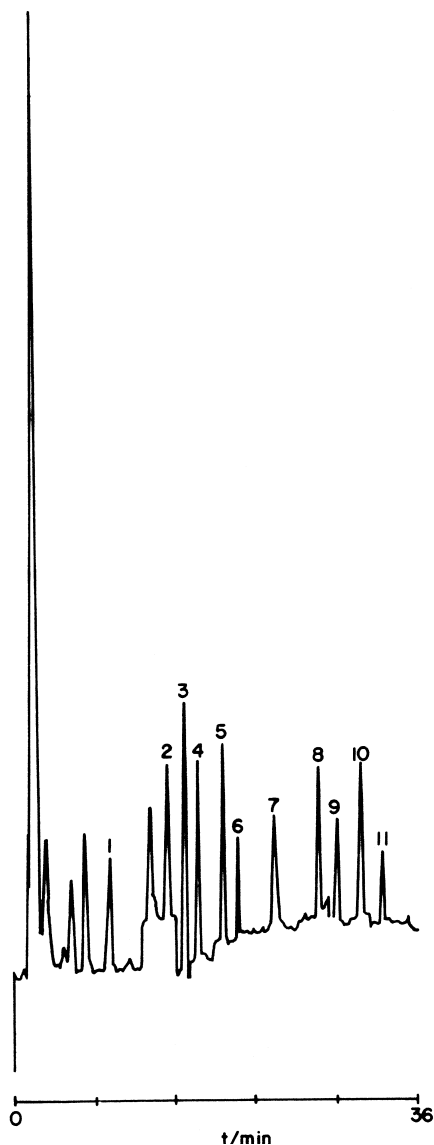
Figure 2. Chromatogram of a spiked toasted bread sample with PAHs standard. Conditions: Hypersil Green PAH (100 x 4.6 mm) column; Temperature, 23°C; Mobile phase, gradient of acetonitrile/water, see Table 1; Flow-rate, 0.8 mL/min; Fluorimetric detection, see Table 2; Injection volume, 20 \mu L. Peaks: 1, Naphthalene; 2, acenaphthene; 3, phenanthrene; 4, anthracene; 5, fluoranthene; 6, pyrene; 7, chrysene; 8, B[e]p; 9, B[a]p; 10, Db[a,h]a; 11, B[ghi]p.
